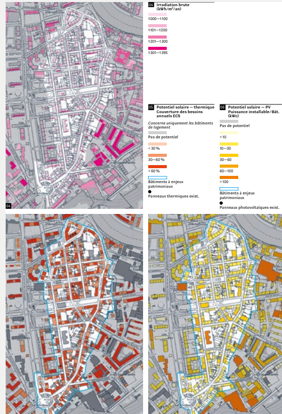
Solkultur methodology to maximise solar energy with high-quality Baukultur . Irradiation plan for Carouge, Switzerland, 2019. © FOC
